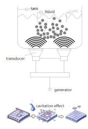
Ultrasonic cleaning is on based on the cavitation effect caused by high frequency ultrasonic wave vibration signal in the fluid. Microscopic bubbles are formed, and they implode violently causing the cavitation which create an intense scrubbing action on the surface of the item being cleaned. The bubbles are small enough to penetrate microscopic crevices, cleaning them thoroughly and consistently.
